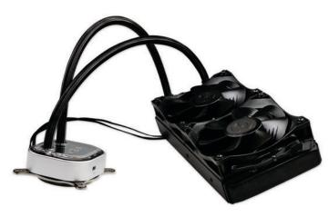
The EVGA CLC 240mm All-In-One RGB LED CPU Liquid Cooler has arrived! This new liquid cooler from EVGA gives you incredible performance, low noise, and robust software controls. The full copper waterblock pulls the heat from your CPU to the radiator, where newly designed fans, featuring Teflon Nano Bearings, effortlessly disperse the heat.
